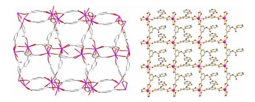
Six new heterometallic coordination polymers have been synthesised by reactions of a pyridyl- and carboxylate-containing ligand 5-(isonicotinamido)phthalic acid with Cu(II)/Co(II) and Ln(III) salts. Complexes 1-3 display twofold interpenetrated 3D structure, while 4-6 display non-interpenetrated 3D network. The luminescent and magnetic properties of the complexes are investigated.
